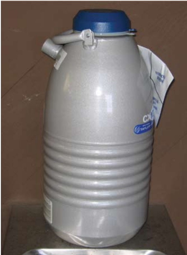
Figure 1. Liquid nitrogen tank.
